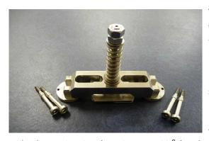
To glue the studs on the inner side of the blade root, the technicians are provided with a dedicated battery operated tool for quick mounting and accurate mutual positioning. Prior to bonding of the studs, the specific areas of the blade are grinded using the stud mounting tool. For the mounting of the studs an adhesive was selected
