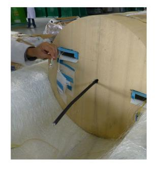
The acquisition module monitors pairs of DTGs along the blades. Fibers can be embedded or attached directly to the surface and are placed at high fatigue areas. An optical technique is preferred because of its high linearity, reliability and long life without maintenance.
