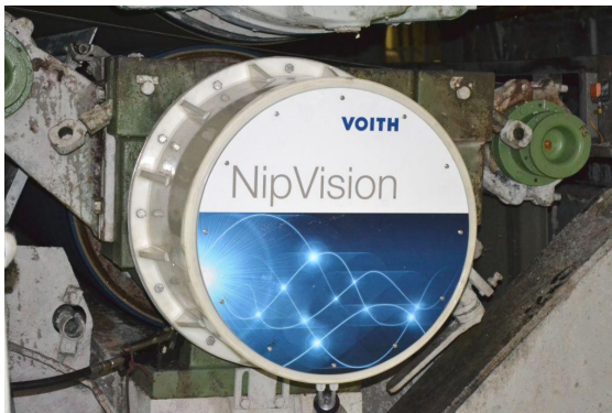
Fig. 6 Rotating fiber optic Bragg grating sensor system NipVision at press section roll axis of paper machine
