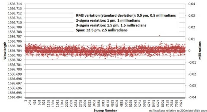
Figure 3. Stability of the laser wavelength referenced to a H<sup>13</sup>CN gas absorption cell at 100 torr (dBm Optics inc.). Plot shows a total of 8000 laser sweeps over a 30 minute period. Sweep rate was 118 kHz.
