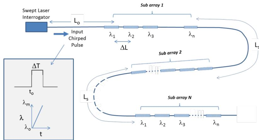
Figure 1. Schematic of the Swept Wavelength to Time Domain Reflectometry Scheme for FBG arrays
