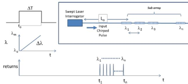
Figure 2. Illustration of the arrival times of the FBG returns for the first sub-array in the system of Figure 1.
