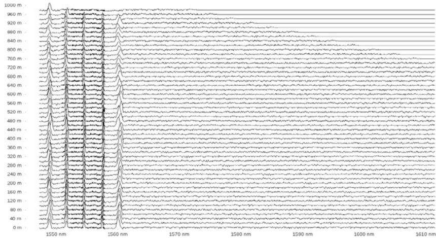
Figure 4. Return signal from the array of 250 FBGs arranged in 50 sub-arrays of 5 FBGs each. The system design would accommodate 20 FBGs in each sub array for a total capacity of 1000 FBGs.
