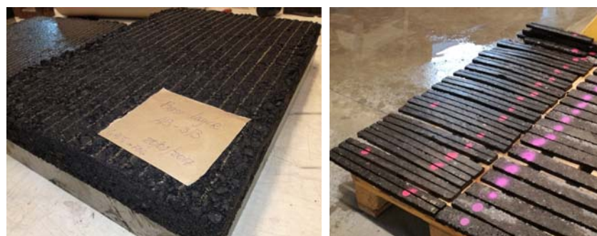
Figure 4. Prefabricated asphalt (AC-14) specimens with grooves for preparation of FBG embedment.
