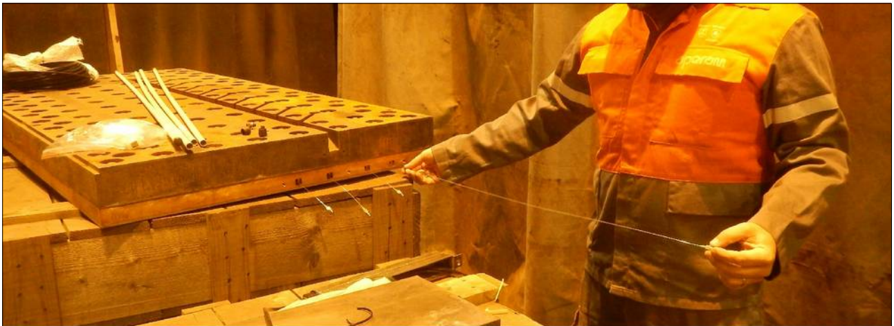
Fig.6 – Installation the fibers into the copper.
