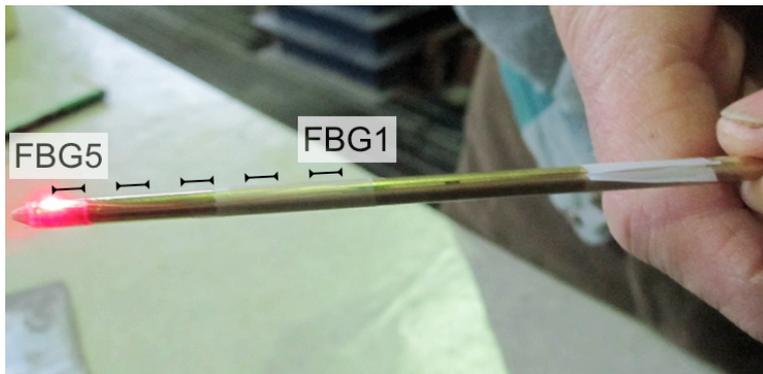
DTG array including 5 sensors, with 1 cm spacing and 0.5 cm active length. Bare fiber with 125  $\mu\text{m}$  thickness, with no additional protection, patched on a 4-mm ablation device, with 1 cm active length.
