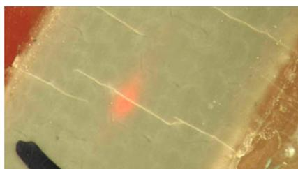
Fig. 13 Micro-crackings in Redux® packaging.
